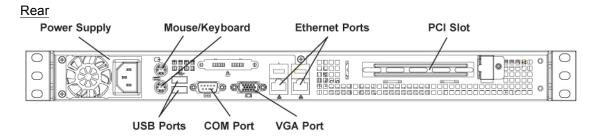
The external USB ports support the vtAlpha and vtVAX license key. The vtLicense-RM2 has four (4) USB ports in the position labeled "PCI slot" in the diagram above, picture below.
