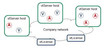
Each vtServer host may run one or more vtAlpha and vtVAX instances simultaneously. These instances may be either production or 'disaster recovery' instances. Additional host hardware can be provisioned to allow these instances to failover to backup systems, either with manual intervention or automatically (e.g., VMware vMotion). When used with vtLicense servers, the vtAlpha and vtVAX instances will automatically discover their licenses across the network, allowing for automatic host transitions.
